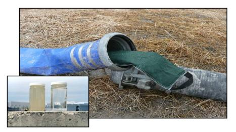
Dungeness Environmental invented *Passive Treatment* with Chitosan Lactate cartridges. Simply anchor the ChitoVan LC cartridge in flowing dirty water and it will convert to a slow-dissolving gel. As it dissolves it automatically doses the water causing sediment particles to coagulate. After coagulation the water may be gravity settled, biofiltered, infiltrated, sand filtered or filtered by dewatering bag.
